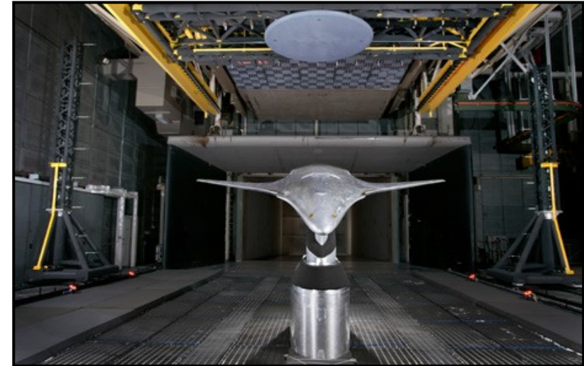
Wind tunnel test setup featuring the Hybrid Wing Body model (inverted), with 97-microphone phased array (top) and microphone tower (left).
